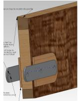
Front spar design and build up. Most parts that are bonded with epoxy. The grey in this part is the metal ears, all other parts are wood as shown.
