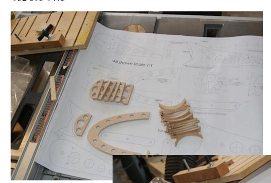
Above– parts cut to pattern being checked to the prints.
